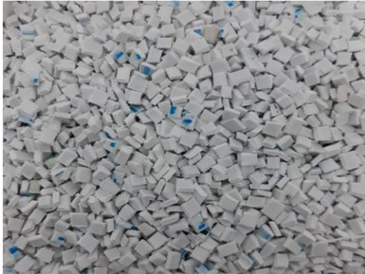
Gambar 1 Agregat halus PVC
